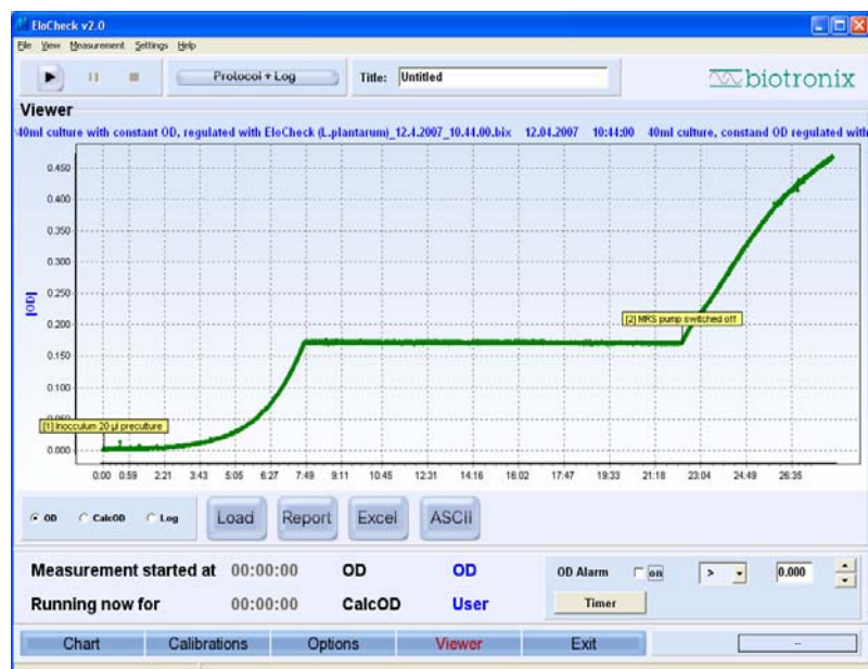
EloCheck screenshot of a fermentation of L. plantarum in MRS medium: After reaching a specified optical density, fresh medium is added automatically so that the biomass concentration was stable over 14 h. The medium pump was switched off in the last phase of this cultivation.
